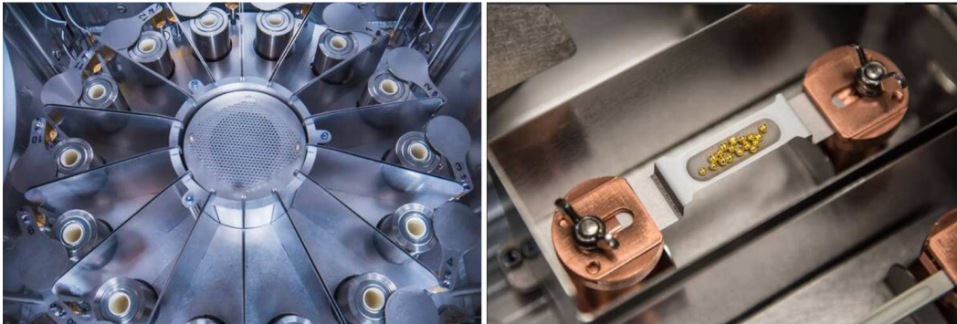
Figure 4-9 LUXEL furnaces (left) and an ohmic resistance boat (right) [19].
