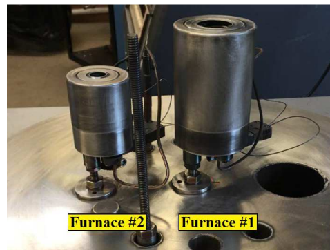
Figure 4-14 E6-TE with two LUXEL furnaces to evaporate CdSe with Se flux.
